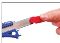
3. Carefully take out the snap blade and replace with a new one
