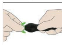
Grasp the head guard and handle firmly while pressing thumb down on the locking tab.
