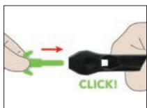
Important: Insert the new head until the locking tab clicks in place. The head should NOT pull back out without depressing the locking tab.
