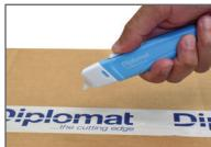
1. Push blade slider forward to extend blade
