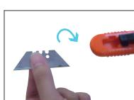
5. Rotate the blade if needed or replace with new blade
