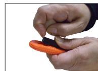
3. Lift the black slider upwards
