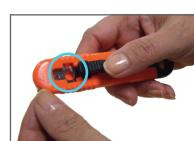
6. Load and place blade until centre hole aligns with rectangular slot
