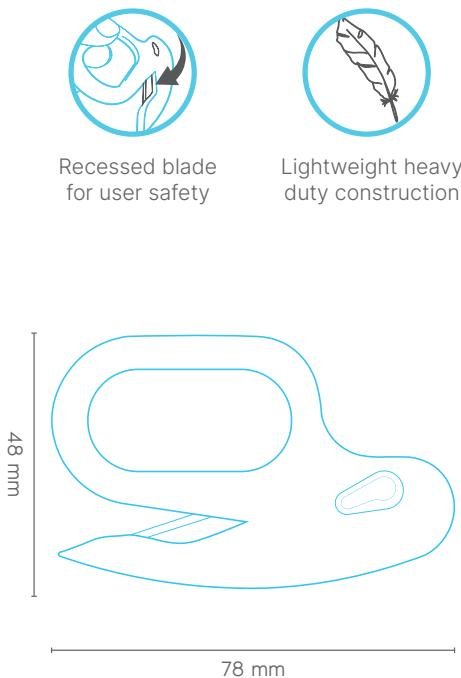
The Diplomat A23HD Heavy Duty Safety Slitter is the perfect ergonomic safety cutter for heavy duty applications. Its large recessed blade design ensures user friendly and is ideal for cutting thicker materials or multiple layers with precision cutting. It is compact and lightweight which delivers maximum cutting capability with minimum effort, making this the ideal tool for multiple cutting tasks.
