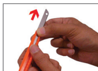
2. Carefully pull out blade & reload with a new fresh blade
